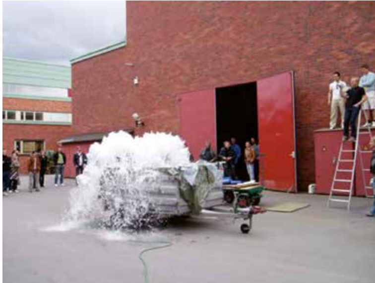
Flood pump (120 litres/s) developed by students, Integrated Product Development.
