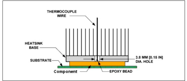
Figure 13-7. Technique for Measuring Tcase with 90° Angle Attachment
