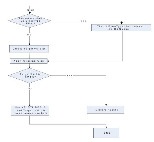
Figure 7-3. Receive Queuing Flow (Virtualization)
