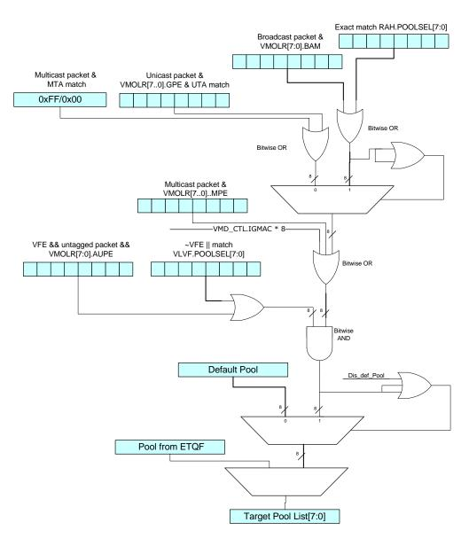
Figure 7-22. Pool List Selection - Replication Enabled
