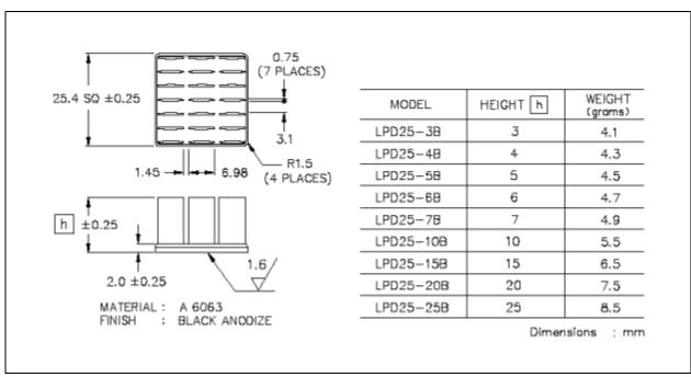
Figure 13-4. 7mm Height Passive Heat Sink (Alpha Novatech, Inc. PN: LPD25-7B)
