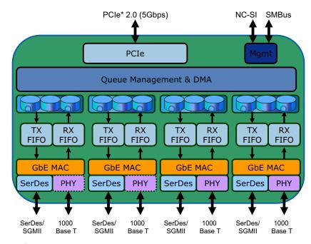
Figure 1-1. Intel<sup>®</sup> 82580 Quad/Dual GbE LAN Controller
