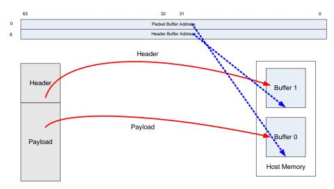
Figure 7-10. Header Splitting
