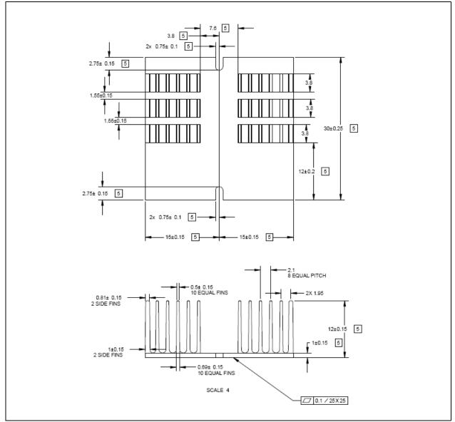
Figure 13-1. Rose City 12 mm Height Passive Heat Sink
