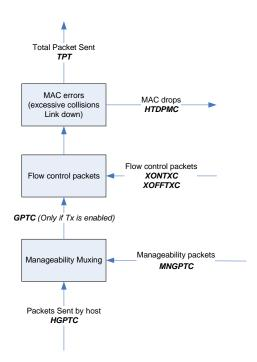
Figure 7-27. Transmit Flow Statistics
