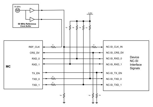
Figure 12-7. NC-SI Connection Schematic: Single-Drop Configuration
