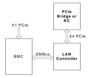
Figure 10-1. 82580 to BMC Connectivity Through a SMBus Connection
