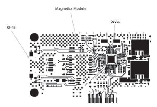
Figure 12-2. Layout for Discrete Magnetics
