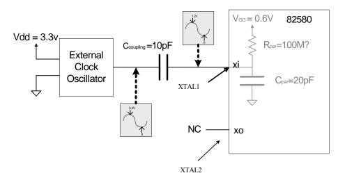
Figure 11-10. External Clock Oscillator Connectivity to the 82580
